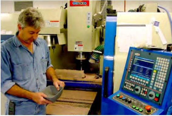
Breville making rapid prototypes of designs using CNC Milling, photo courtesy of Breville
